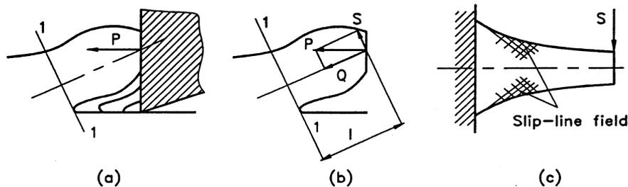
Fig. 6. The interaction between the tool rake face and the chip: (a) penetration force  $P$  acting on the chip; (b) two components of the penetration force, namely, the compressive force  $Q$  and the bending force  $S$ ; (c) plastic deformation of an elastoplastic cantilever having a curved contour by the bending force  $S$ .
