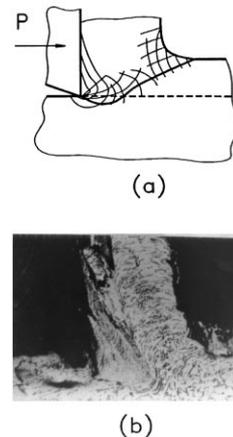
Fig. 9. Shape of the lower boundary of the deformation zone: (a) as modeled by superposition of the slip-line fields due to bending; (b) a 'frozen' picture of the deformation zone obtained using a quick-stop device ( $\times 60$ ).
