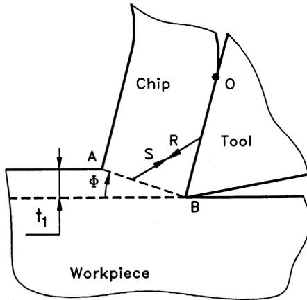
Fig. 1. Configuration of the metal cutting mechanism used in the development of chip formation theory by previous investigators.
