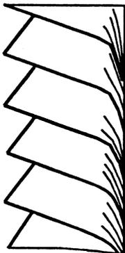
Fig. 8. Structure of the continuous fragmental chip.
