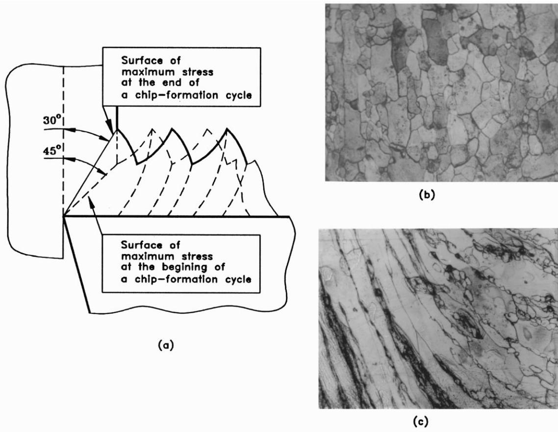
Fig. 10. Model of chip formation reconstructed using experimental results obtained in the cutting of a nickel-based high alloy: (a) a variation of the location of the surface of maximum combined stress within a cycle of chip formation; (b) chip structure at the beginning ( $\times 125$ ); (c) chip structure at the end ( $\times 125$ ) of a chip-formation cycle.
