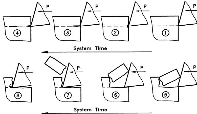
Fig. 3. System consideration of the chip formation in the cutting of a brittle material. The cutting tool has a positive rake angle.
