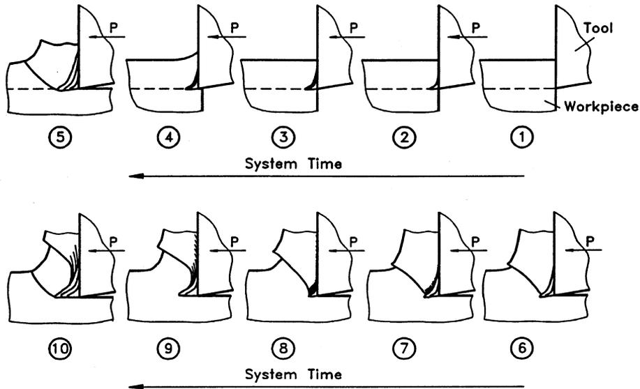
Fig. 7. System consideration of chip formation in the cutting of ductile materials.
