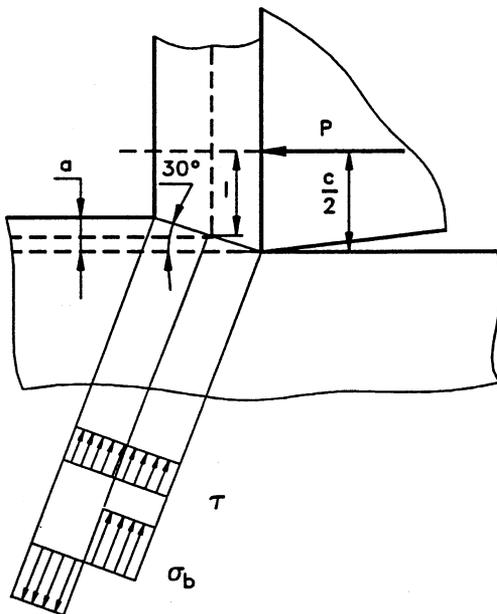
Fig. 11. Model of the cutting mechanism used for the derivation of the analytical expression for the bending stress on the surface of maximum combined stress.
