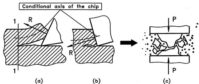
Fig. 4. Two models of chip formation for the machining of brittle materials: (a) the direction of the force resultant  $R$  intersects the conditional axis of the formed chip-cantilever; (b) the direction of the force resultant  $R$  does not intersect the conditional axis of the formed chip-cantilever.
