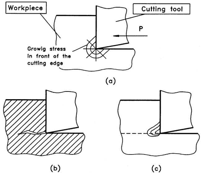
Fig. 2. The cutting tool starting to advance into the workpiece.
